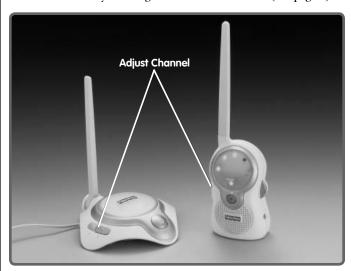
Set transmitter channel switch to same channel as receiver.
